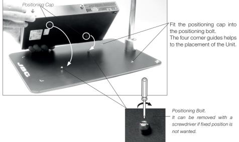
The position of the PHS can be fixed on the RWS by means of positioning caps.
