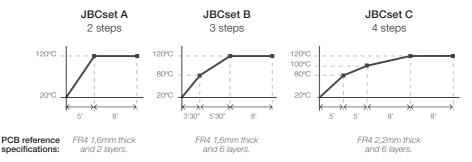
Profiles set using the low position of the PHS-SA Support (28 mm in height between the PCB and the heating area).
